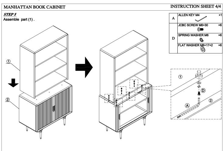
CAUTION: before wall assembling, be sure to match the right screws with the wall type.
