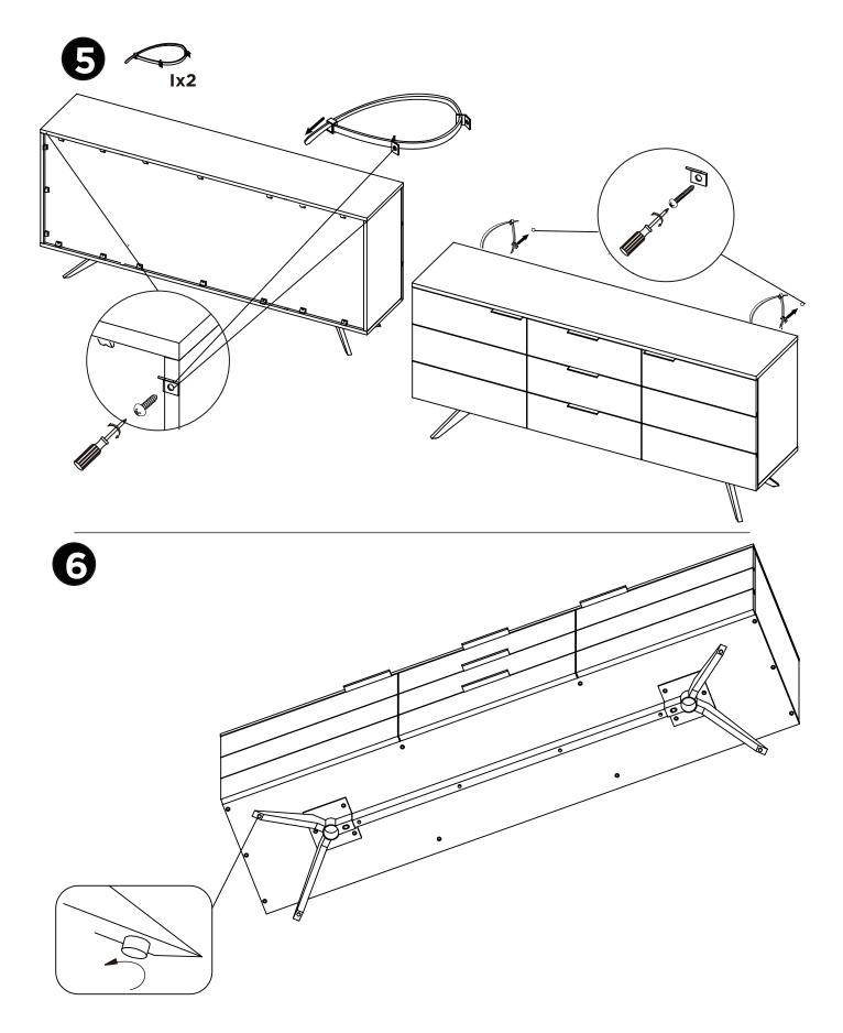
Twist the bolt anticlockwise to adjust the level of sideboard.
