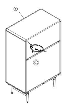
CAUTION: before wall assembling, be sure to match the right screws with the wall type.
